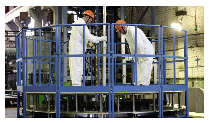
Workers at Rosatom's Research Institute of Atomic Reactors (RIAR) in Dimitrovgrad, 80 kilometers east of Ulyanovsk, work to finish a test assembly of the first reactor for the Center for Nuclear Technology Research and Development, which is currently under construction in the Bolivian city of El Alto situated at 4 kilometers above sea level. The swimming pool WWER reactor developed by RIAR has a capacity of 200kW and operating life of 50 years. **Dmitry Sandimirov / TASS**
