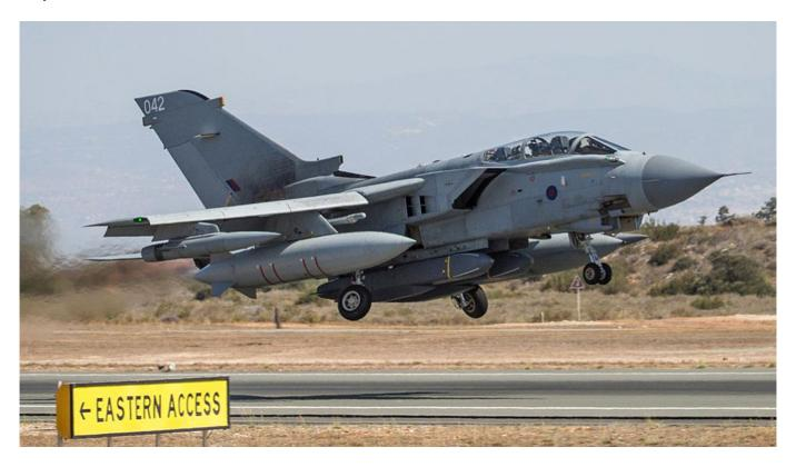
A RAF Tornado GR4 carrying two Storm Shadow missiles under its fuselage. **Davidsmith2014 (CC BY-SA 4.0)**
