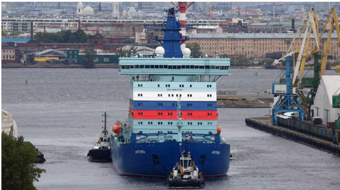
According to its constructors, the Arktika can cut through ice that is 2.8 meters (around 9 feet) thick.
