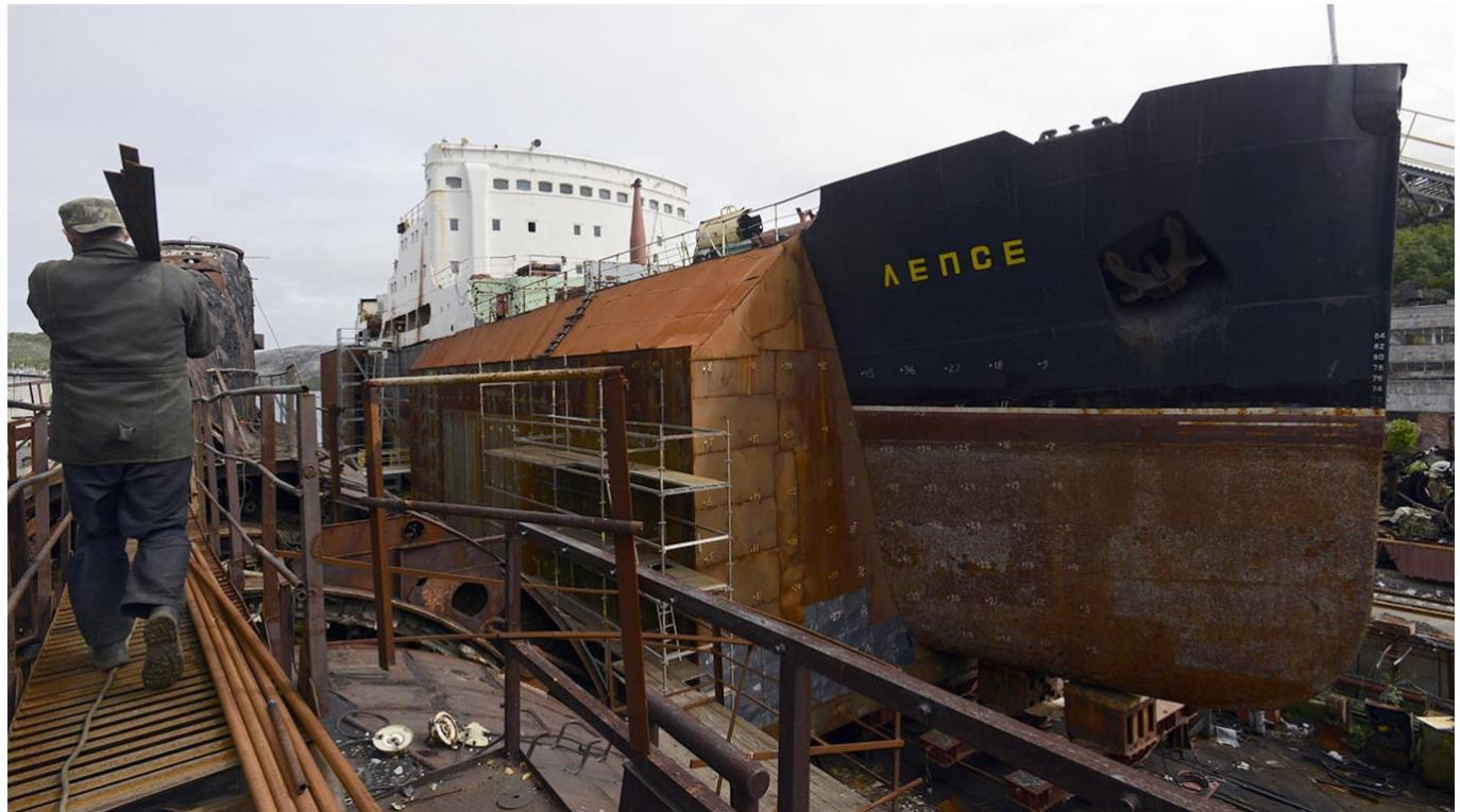
The Lepse held 639 damaged and distorted spent nuclear fuel assemblies when it was taken out of service. **Lev Fedoseyev / TASS**
