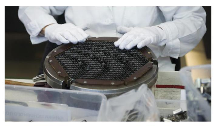
Manufacturing fuel assembly frames for nuclear power reactors at Novosibirsk Chemical Concentrates Plant. **Kirill Kukhmar / TASS**
