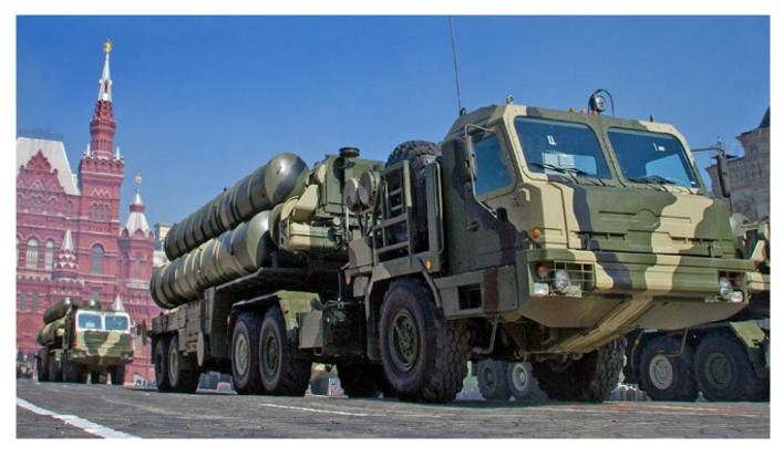
The S-400 is Russia's top of the line air defense system, capable of intercepting targets up to 250 kilometers away.
