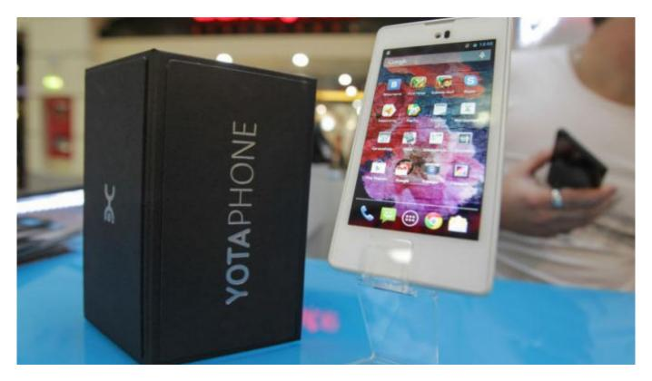
A YotaPhone smartphone, which was first launched in December 2013, has a standard LCD screen on one side, and an e-ink screen on the other side.
