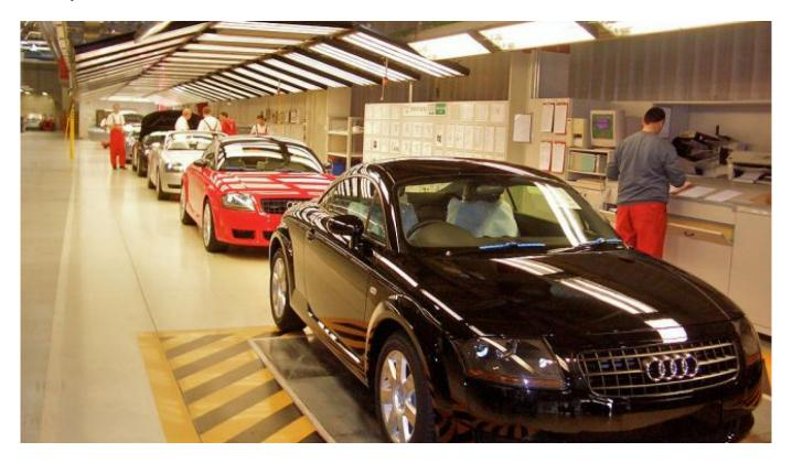
The final inspection of assembled Audi TT's in Gyor, Hungary.
