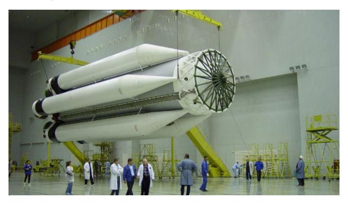
Production floor of the Khrunichev Space Center, where Russia's venerable Proton-M rockets are constructed.
