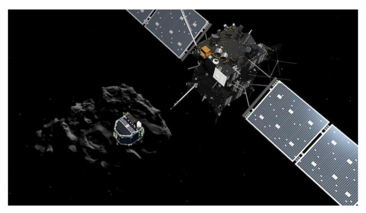
Philae separating from Rosetta and descending to the surface of comet 67P/Churyumov-Gerasimenko.
