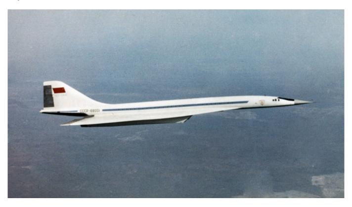
Tupolev Tu-144 supersonic airliner was used to train pilots for the aborted Buran space shuttle program.
