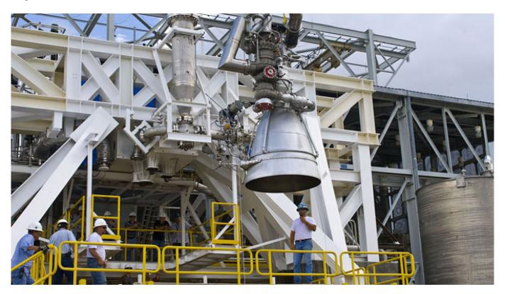
A modified NK-33 engine rocket engine being prepared for installation.
