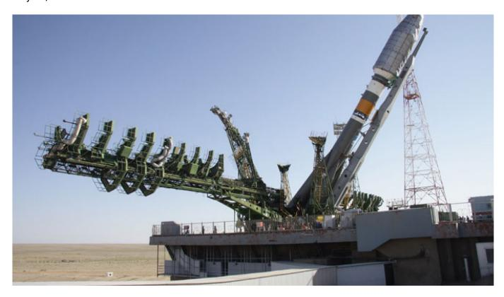
A Soyuz 2.1b rocket, with its visibly larger payload faring, being lifted into launch position at the Baikonur Cosmodrome in June.
