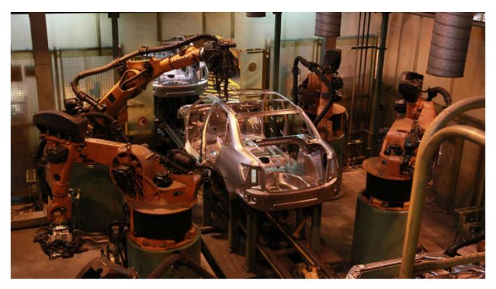
A robotic arm welding the shell of a Lada car on one of AvtoVAZ's production lines in the Volga city of Tolyatti. **Denis Abramov**
