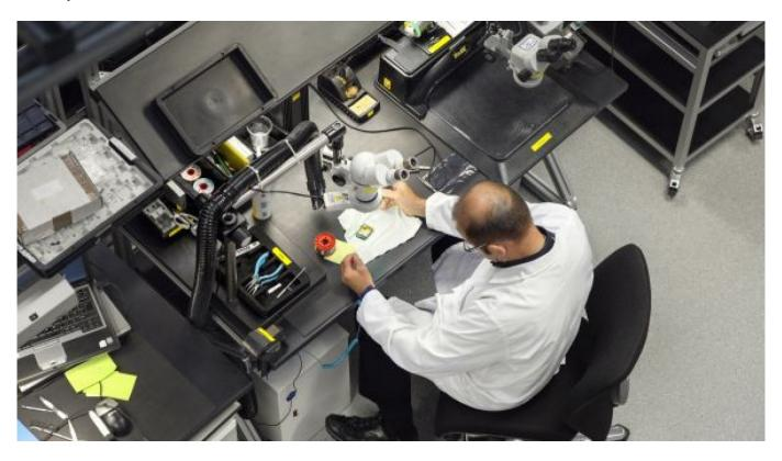
A craftsman making a Vertu mobile phone from grade 5 titanium. They are encased by leather and fitted with sapphire crystal screens.
