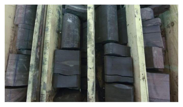
Core samples of the Bazhenov Formation, the world's largest shale oil resource, obtained by exploratory drilling. **Maxim Shemetov**
