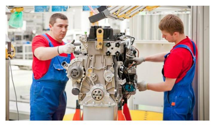
Workers assembling an existing model of an engine at the Yaroslavl Motor Plant.
