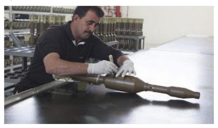
Russian RPG-32 grenade launchers being manufactured at a new plant in Jordan
