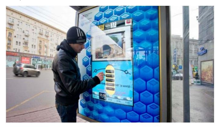
Moscow's first "smart" bus stops have appeared on Tverskaya Ulitsa. The touch panels allow passengers to find out the exact time of the arrival of the bus and - just for Moscow - are covered with a special vandal-proof plastic. **Vladimir Filonov**
