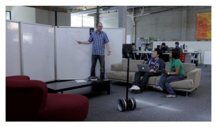
A Double robot, made up of an iPad and a Segway scooter, could be used by students to remotely attend class.
