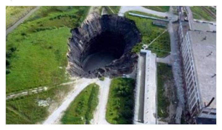
Workers were filling in this sink hole when ground near its edge collapsed.
