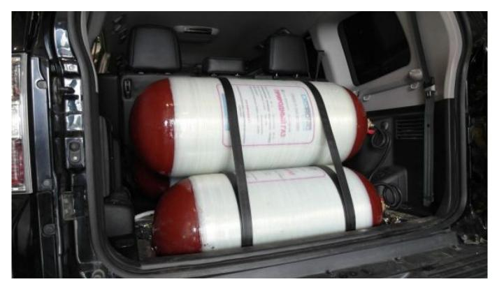
Vehicles that have tanks and engine interfaces can use natural gas, which is less expensive than gasoline.
