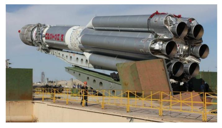
A Proton rocket with an attached Briz upper stage at the Baikonur cosmodrome in Kazakhstan. The company Nesterov headed produces the Briz engines, among other space equipment.
