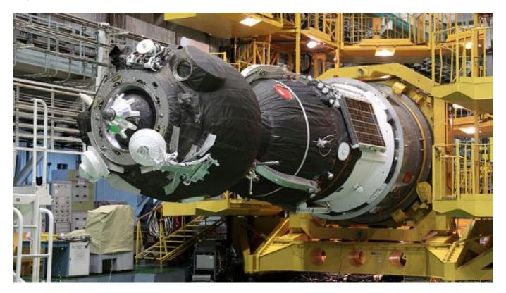
The Soyuz TMA-05M craft in which the astronauts traveled, seen here during pre-launch processing one week before lift-off.
