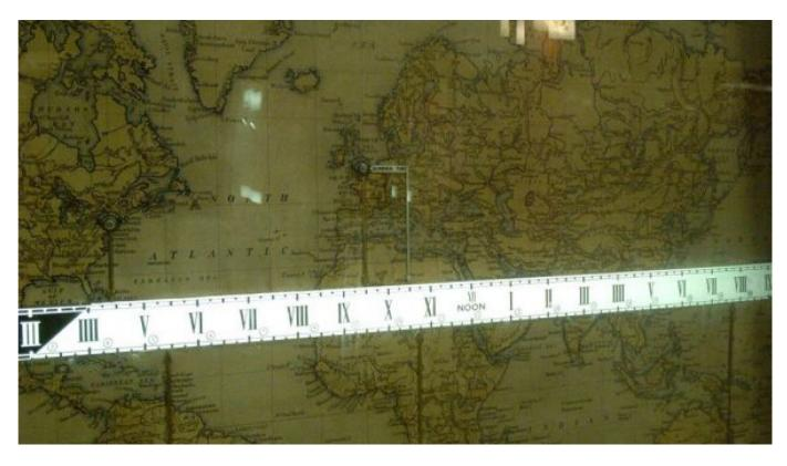
A linear clock in London's Piccadilly Circus metro station. A 24-hour band moves across the static map with a marker to indicate daylight-saving time.
