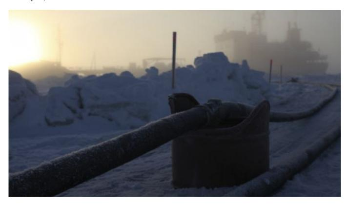
A hose from the Russian tanker Renda being pressure tested at the port of Nome, before fuel pumping starts. **Eric J. Chandler**
