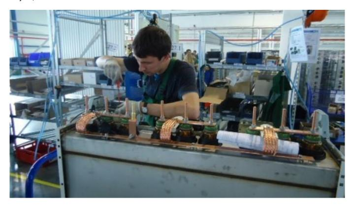
A worker making an RM6 unit at Schneider's new plant, its third in Russia. Roland Oliphant
