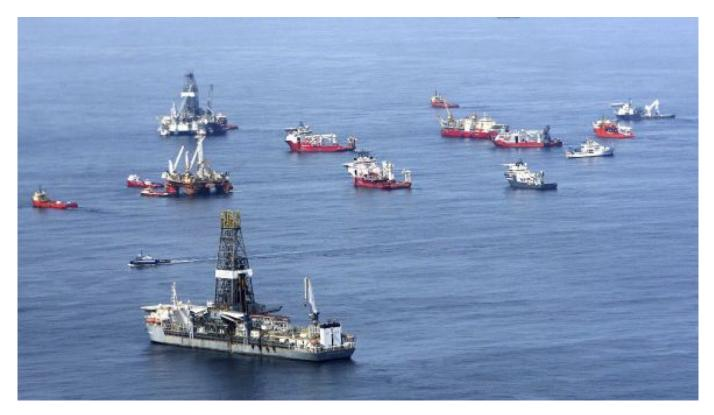
Drill ships and response vessels working in the Gulf of Mexico on a relief well at the site of the Deepwater oil spill. **Sean Gardner**
